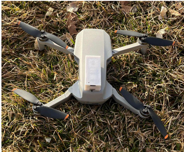
Figure 1: Good placement of module on sample drone. Notice that the module faces upward and is clear of obstructions. This will allow the module to get a GPS fix.
